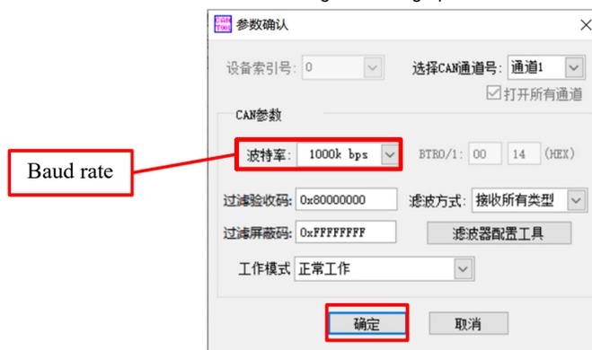
Fig.14 Selecting the baud rate
