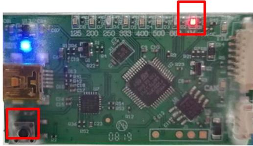
Fig.2 Set baud rate to 1M
