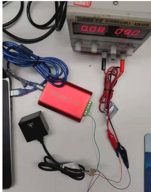
Fig.10 CANalyst connecting TF03-CAN to PC
