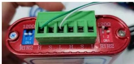
Fig.11 CANalyst and TF03-CAN connection method
