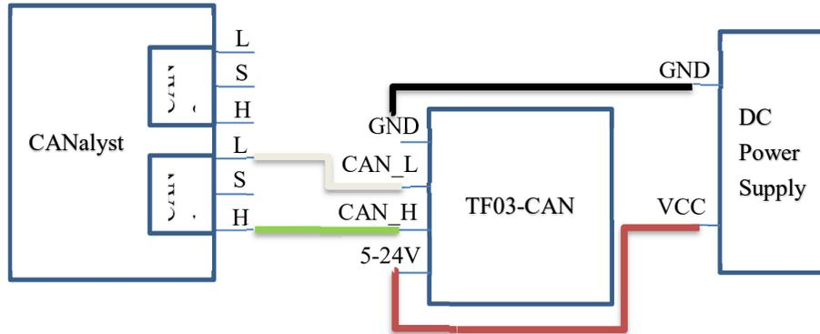
Fig.9 CANalyst connecting TF03-CAN to PC
