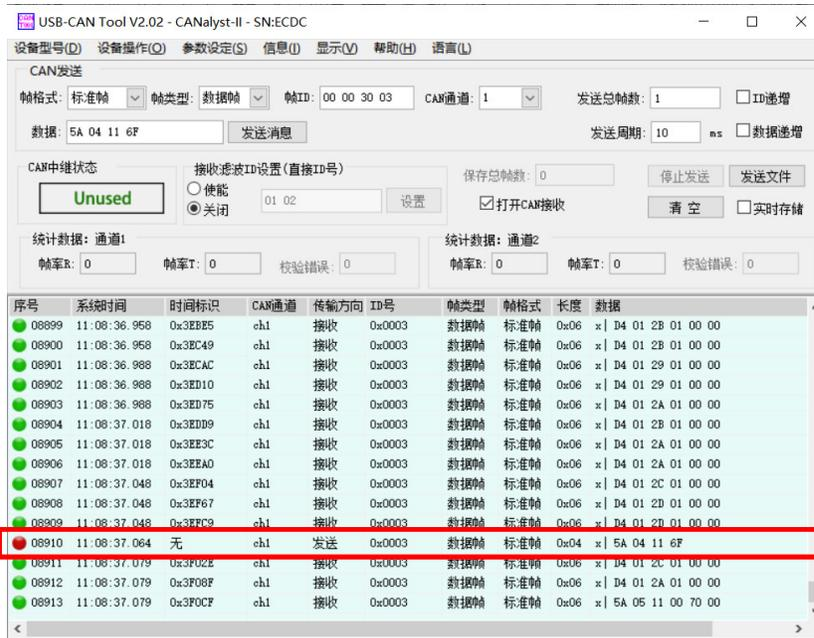
Fig.17 Send "save configuration" command
