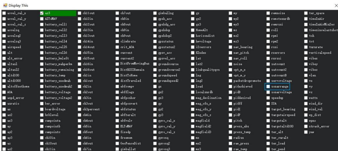
The altitude distance from the LiDAR will be displayed in Sonar Range (meters), see the following picture:
