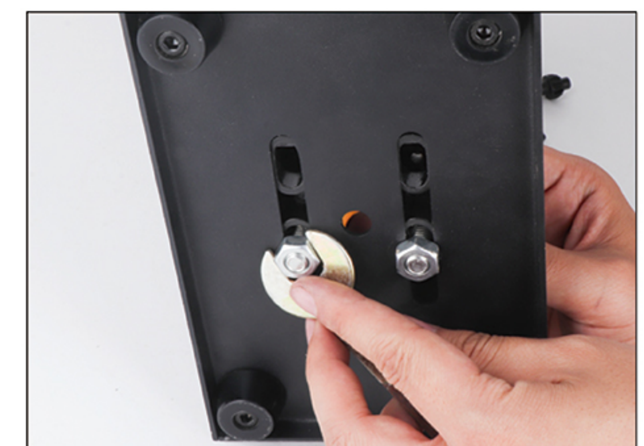
Tighten the hex nut with a wrench to secure it
