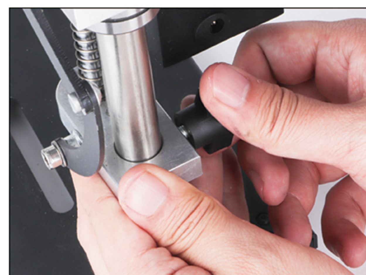
Tighten the lift handle
