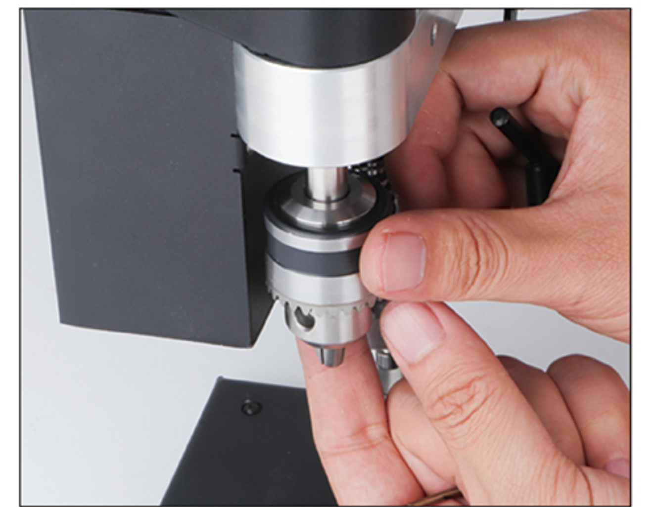
Unscrew the drill chuck
