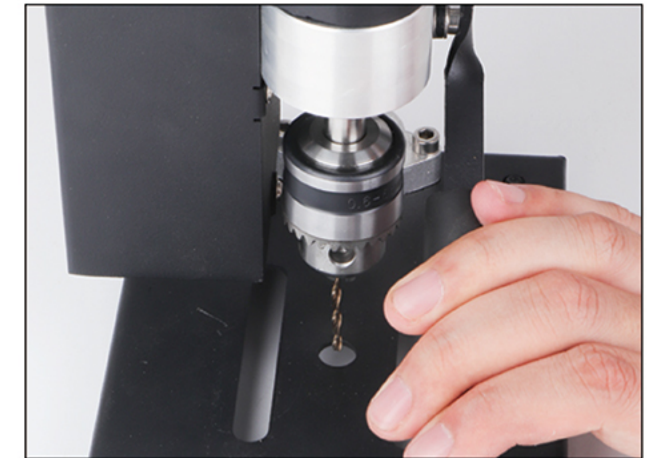
Press the handle down to see if it is aligned with the center hole of the base
