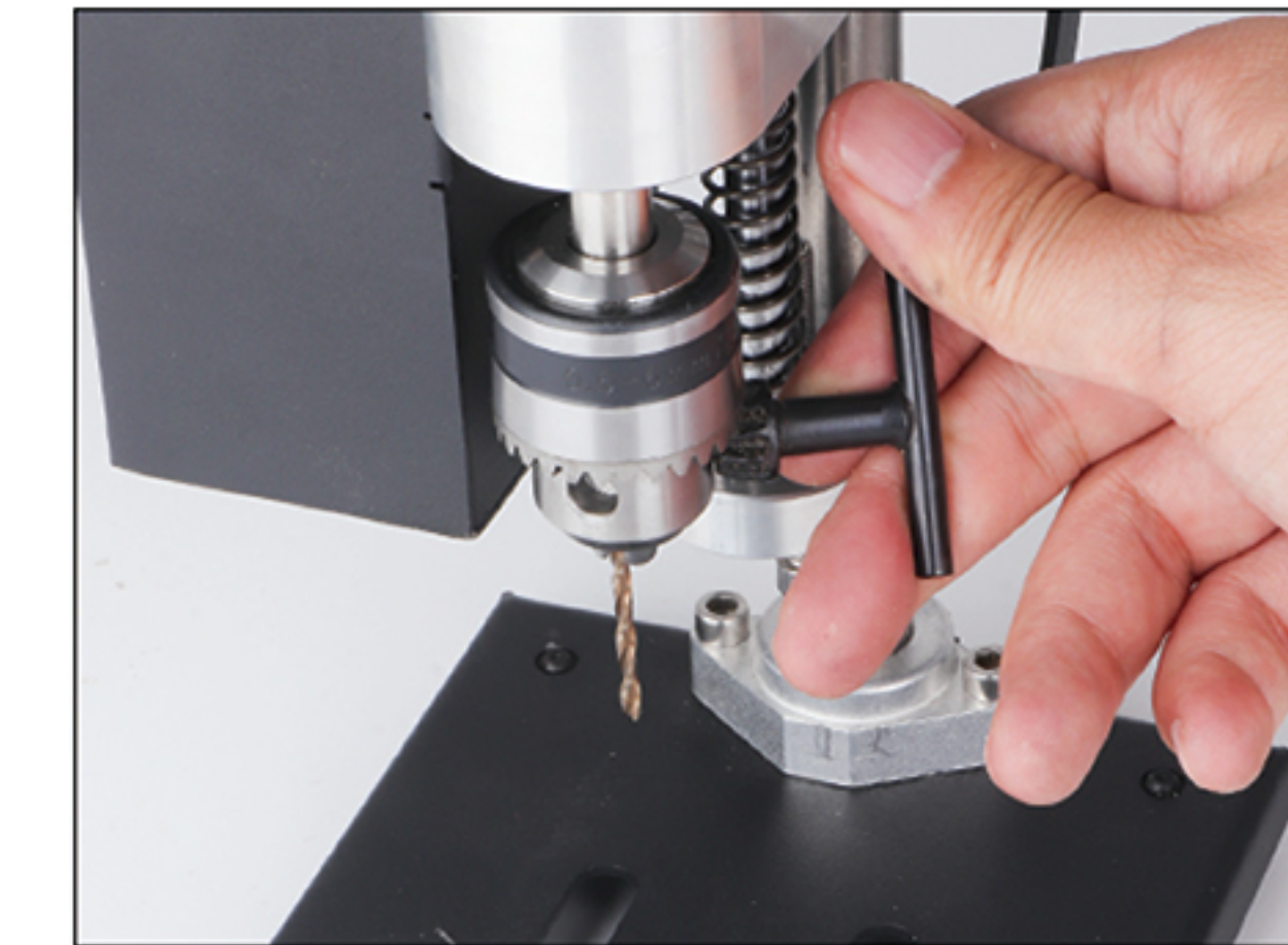
Install the drill bit, use the drill chuck wrench to tighten the lock bit
