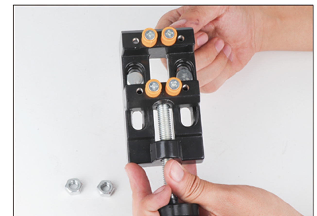
Install the two screws into the slide as shown
