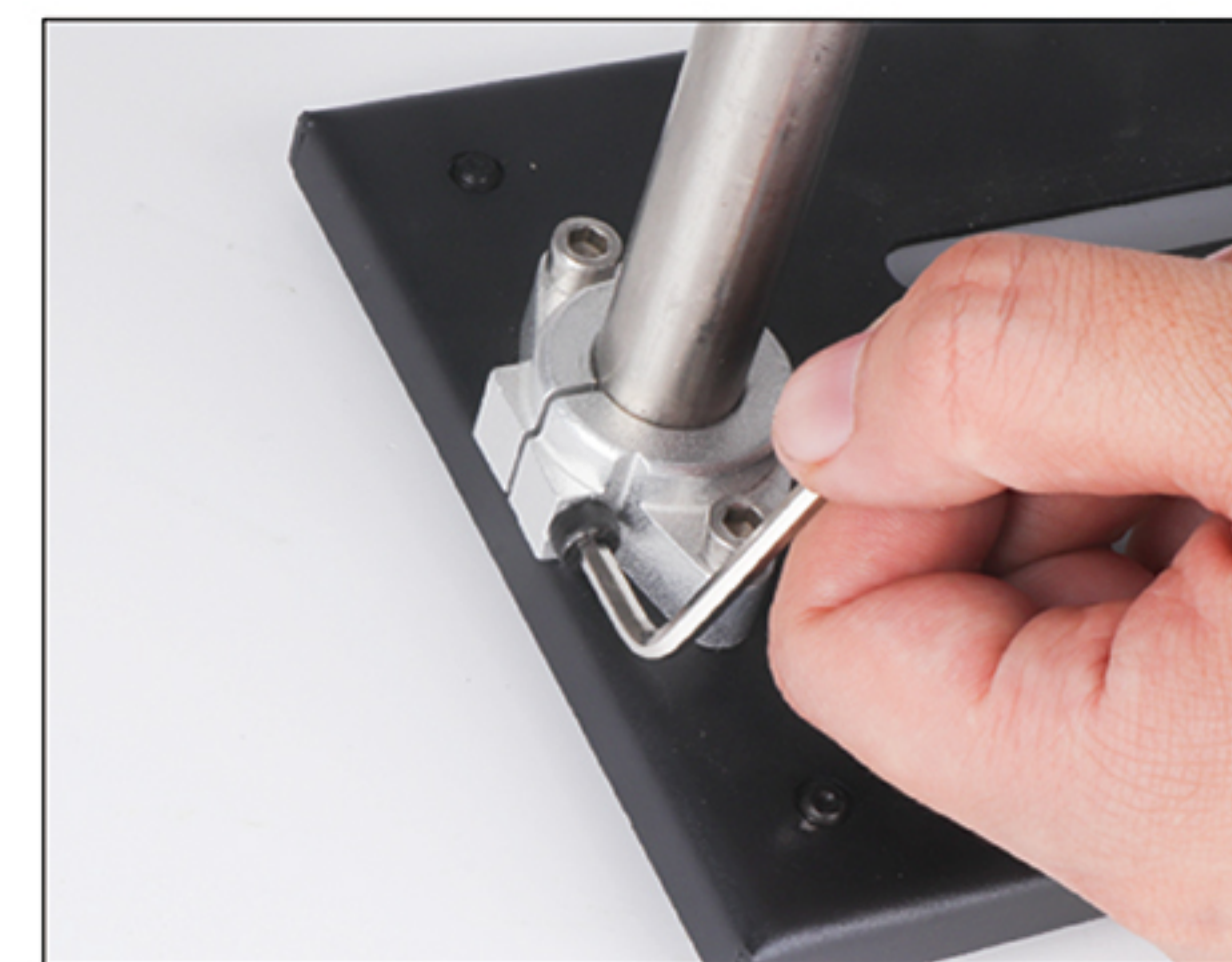
Tighten the screw with an Allen wrench
