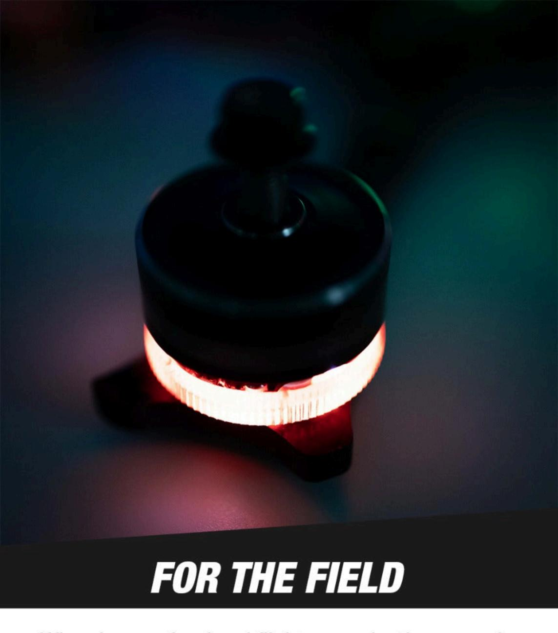
When in a professional flight scenario, the ease of repairing and replacing parts on the field is just as important as the initial design in the aircraft's construction. With the Pulsar series, the motor features a power distribution board for easy desoldering of any wires to make replacement simple.
