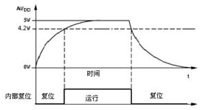
5.8.4 Line voltage drop detection 片内电源供电监视
