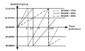
5.4.2 Calculation principle of line cycle energy
