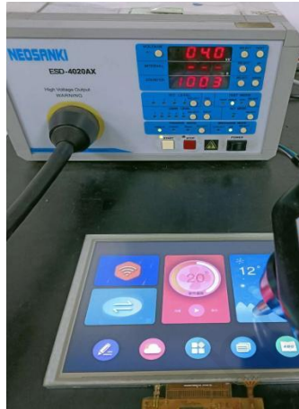
4.1 Electrostatic discharge test
