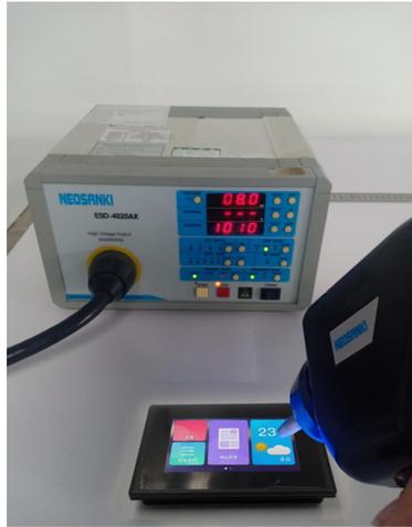
3.1 Electrostatic discharge test
