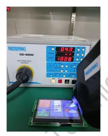
3.1 Electrostatic discharge test
