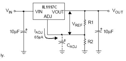
Figure 4. Basic Adjustable Regulator
