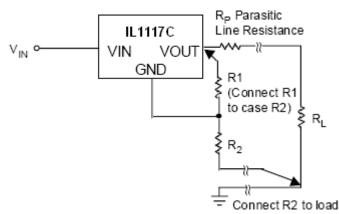
Figure 5. Best Load Regulation Using Adjustable Output Regulator
