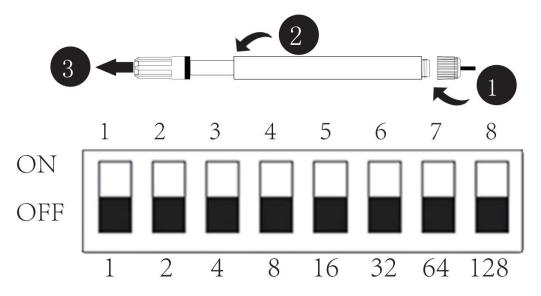
Calculation: the DIP digits1~8 respectively correspond to number 1, 2, 4, 8, 16, 32, 64, 128(as shown in the figure above); Add all the values corresponding to the DIP digits 1-8 dialed to NO, that is the value of the address code. For example:
