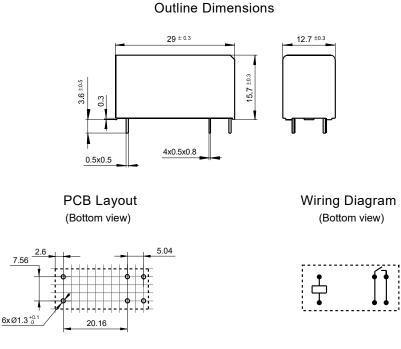
Remark: 1) In case of no tolerance shown in outline dimension: outline dimension <1mm, tolerance should be ±0.2mm; outline dimension >1mm and  $\leq$ 5mm, tolerance should be ±0.3mm; outline dimension >5mm, tolerance should be ±0.4mm.
