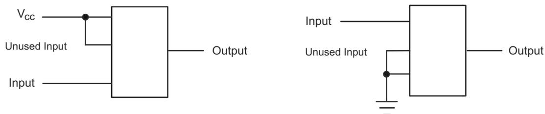
Figure 8-3. Layout Diagram
