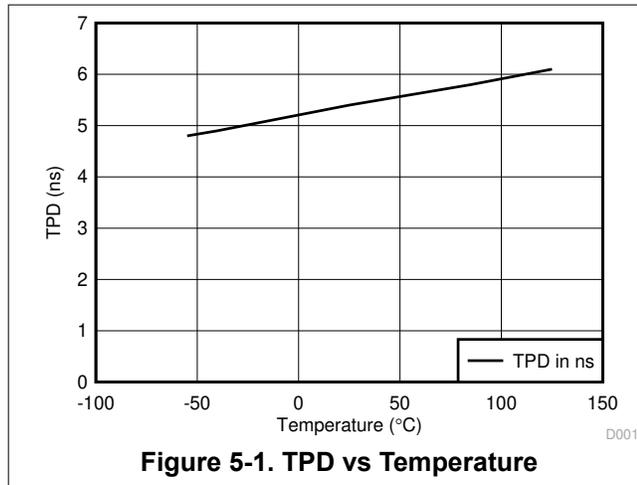
Figure 5-1. TPD vs Temperature
