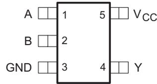
**Figure 4-2. DCK Package 5-Pin SC70 Top View**
