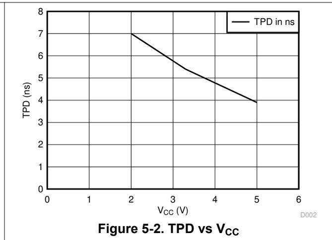
Figure 5-2. TPD vs  $V_{CC}$
