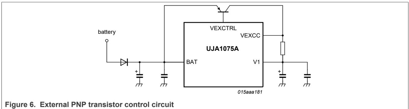
Figure 6. External PNP transistor control circuit
