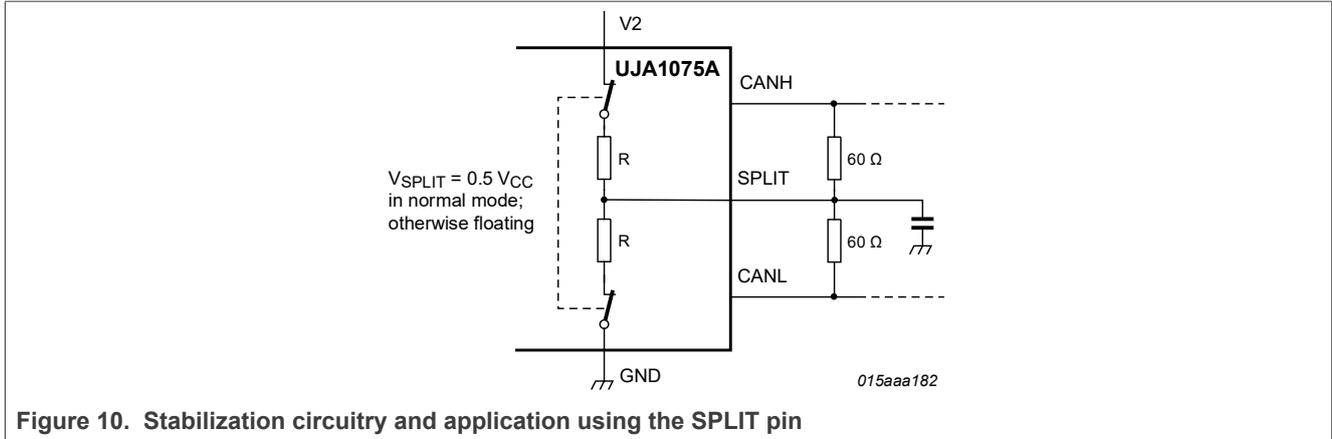
Figure 10. Stabilization circuitry and application using the SPLIT pin
