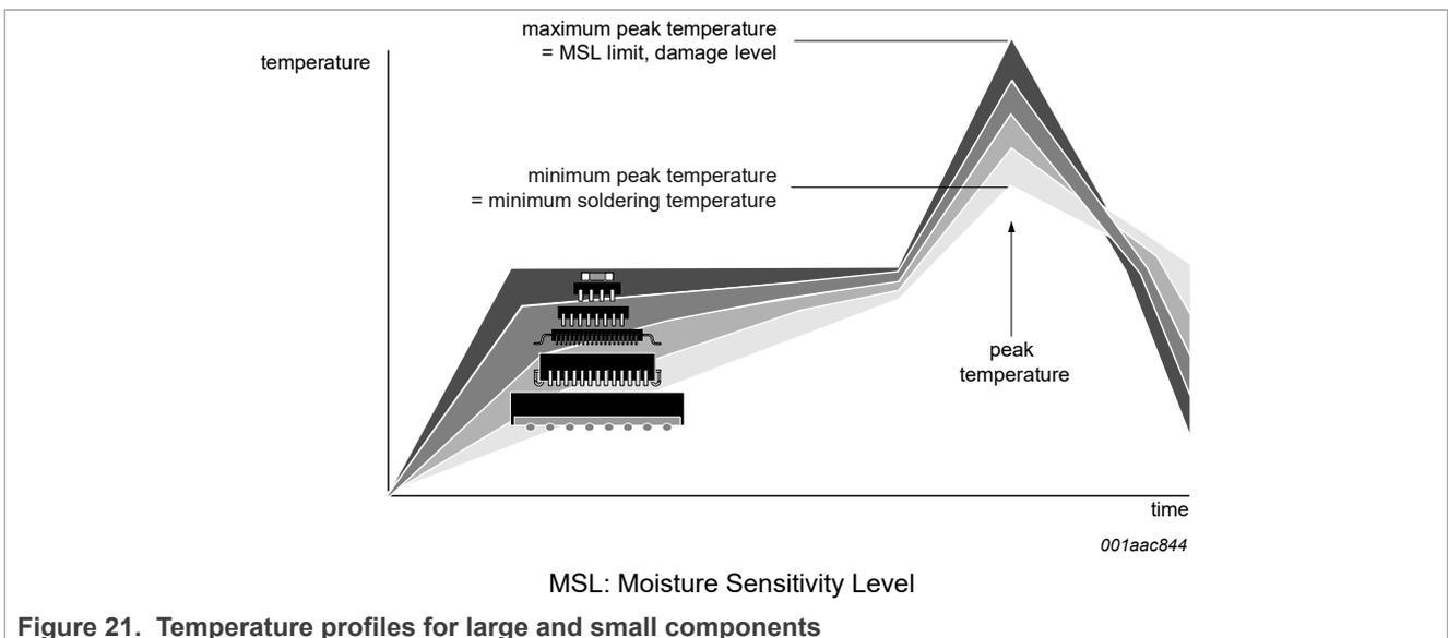
Figure 21. Temperature profiles for large and small components
