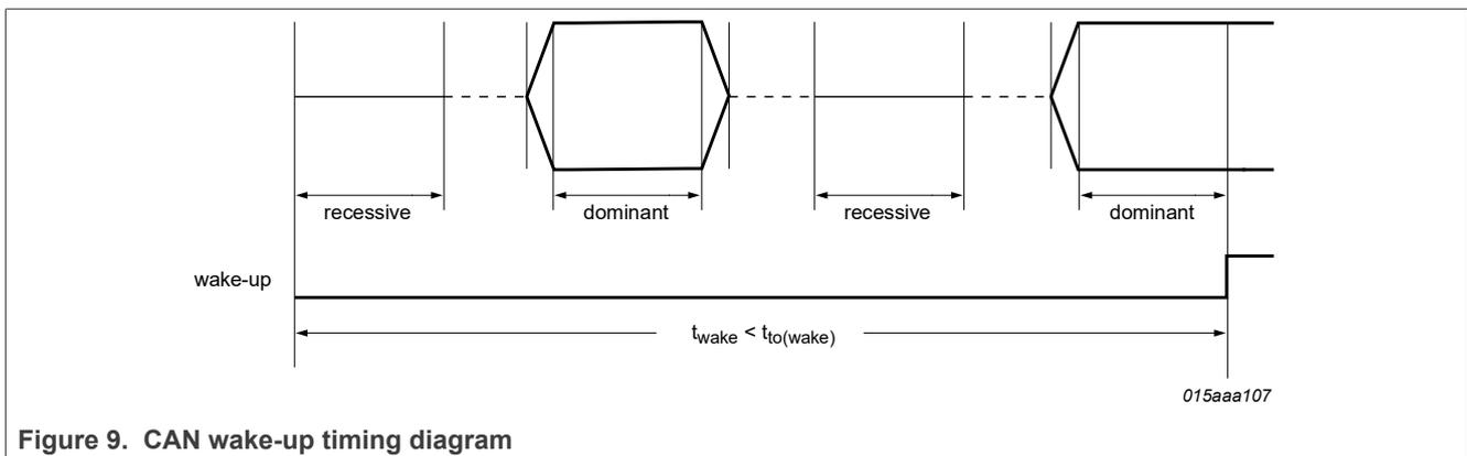
Figure 9. CAN wake-up timing diagram
