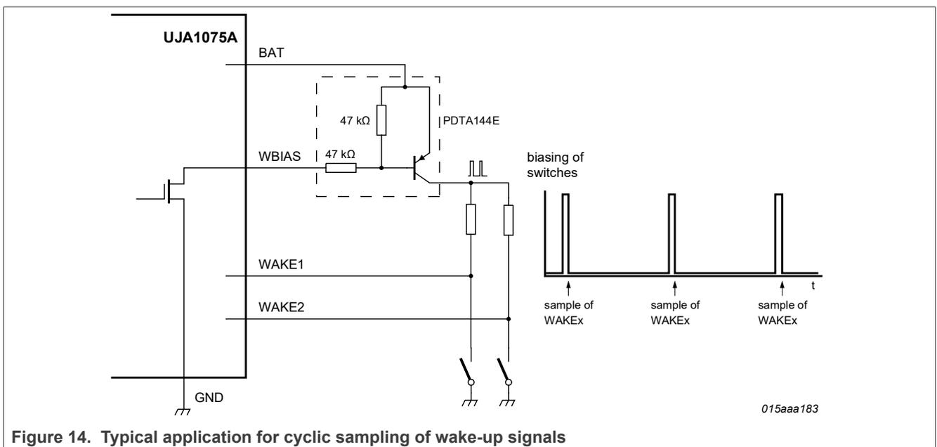
Figure 14. Typical application for cyclic sampling of wake-up signals
