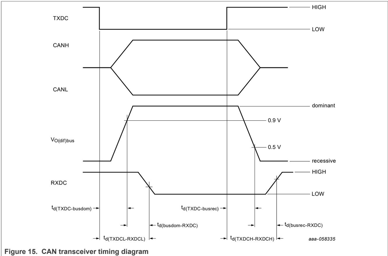
Figure 15. CAN transceiver timing diagram
