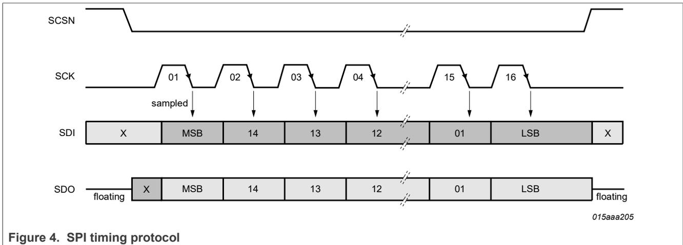
Figure 4. SPI timing protocol
