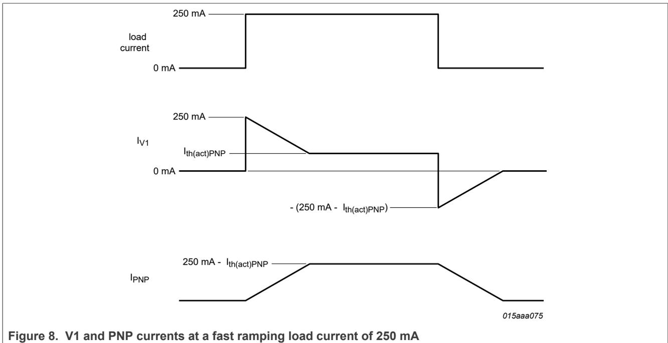
Figure 8. V1 and PNP currents at a fast ramping load current of 250 mA
