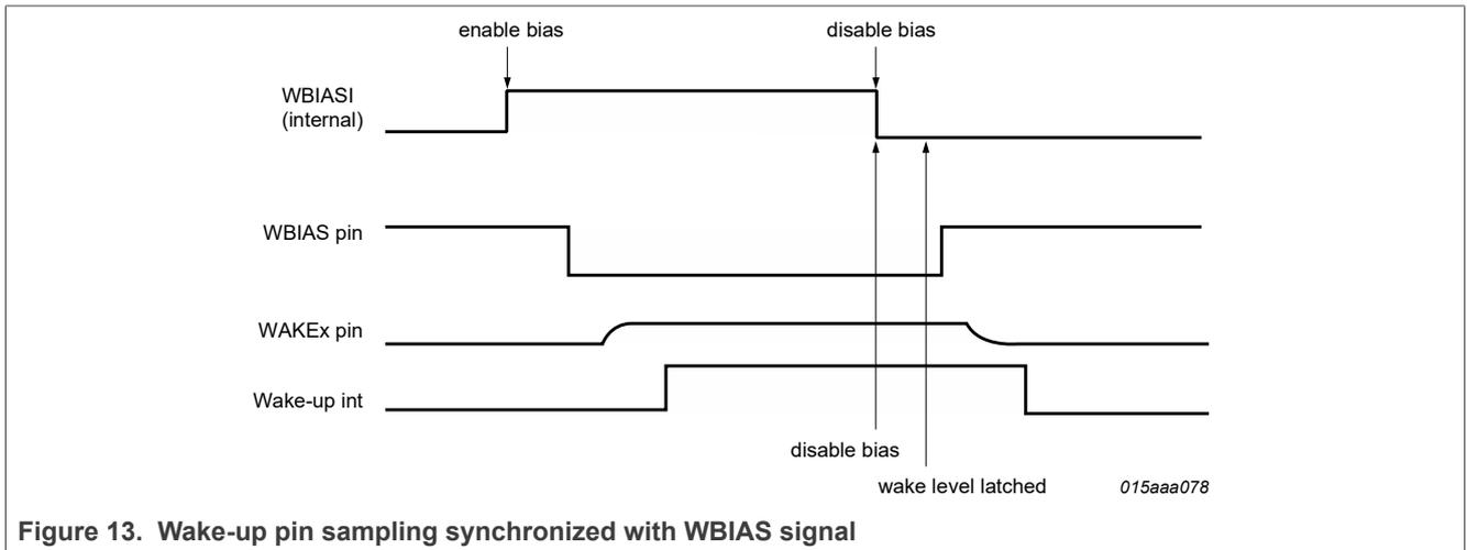
Figure 13. Wake-up pin sampling synchronized with WBIAS signal
