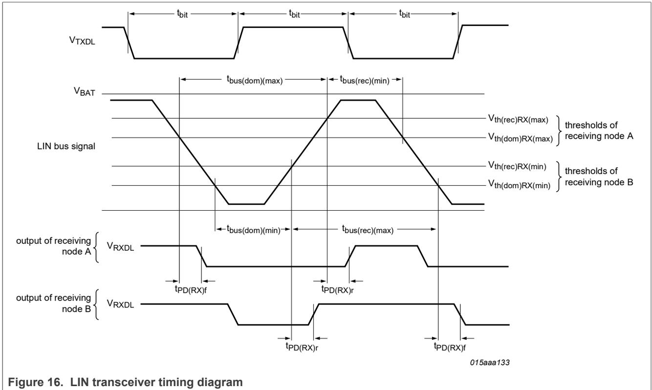
Figure 16. LIN transceiver timing diagram
