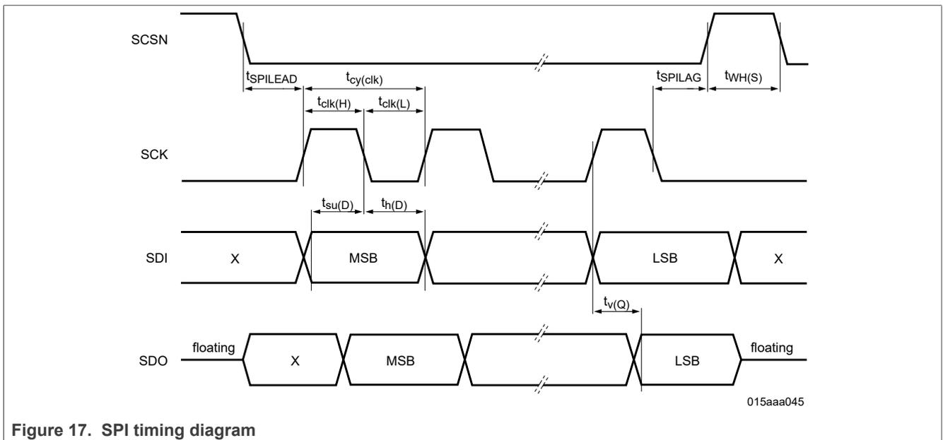
Figure 17. SPI timing diagram
