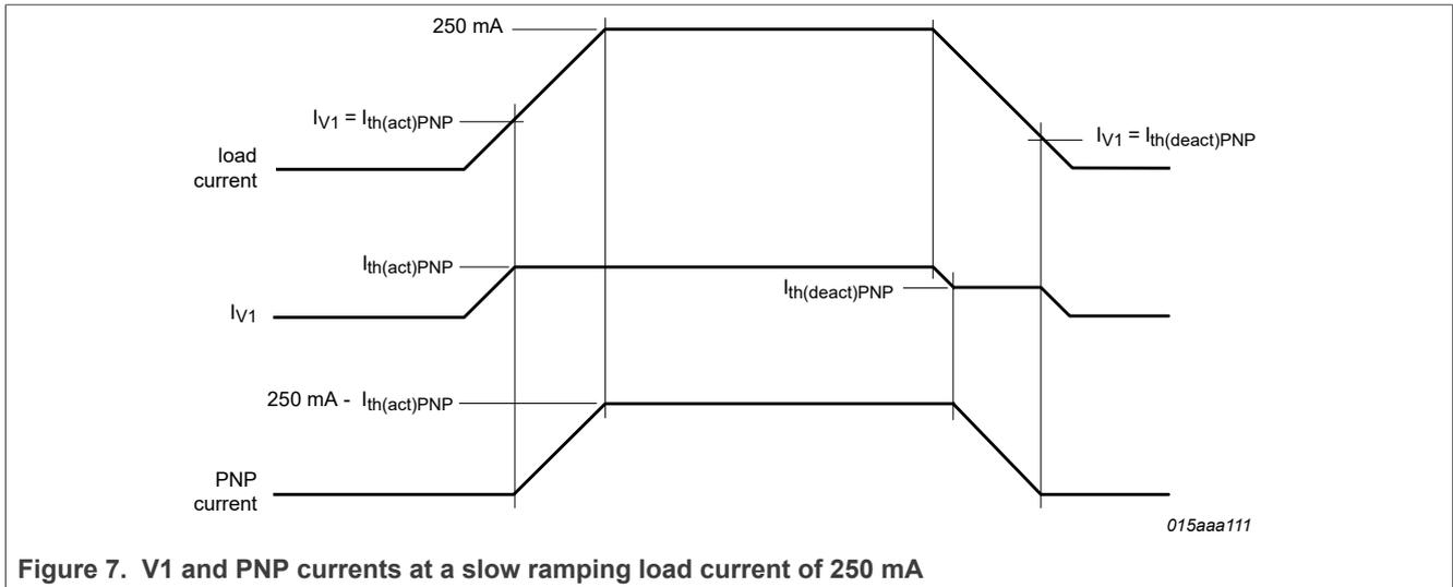
Figure 7. V1 and PNP currents at a slow ramping load current of 250 mA
