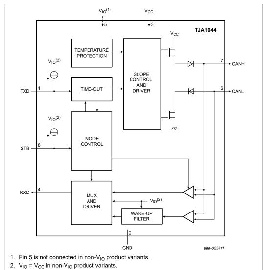
Figure 1. Block diagram
