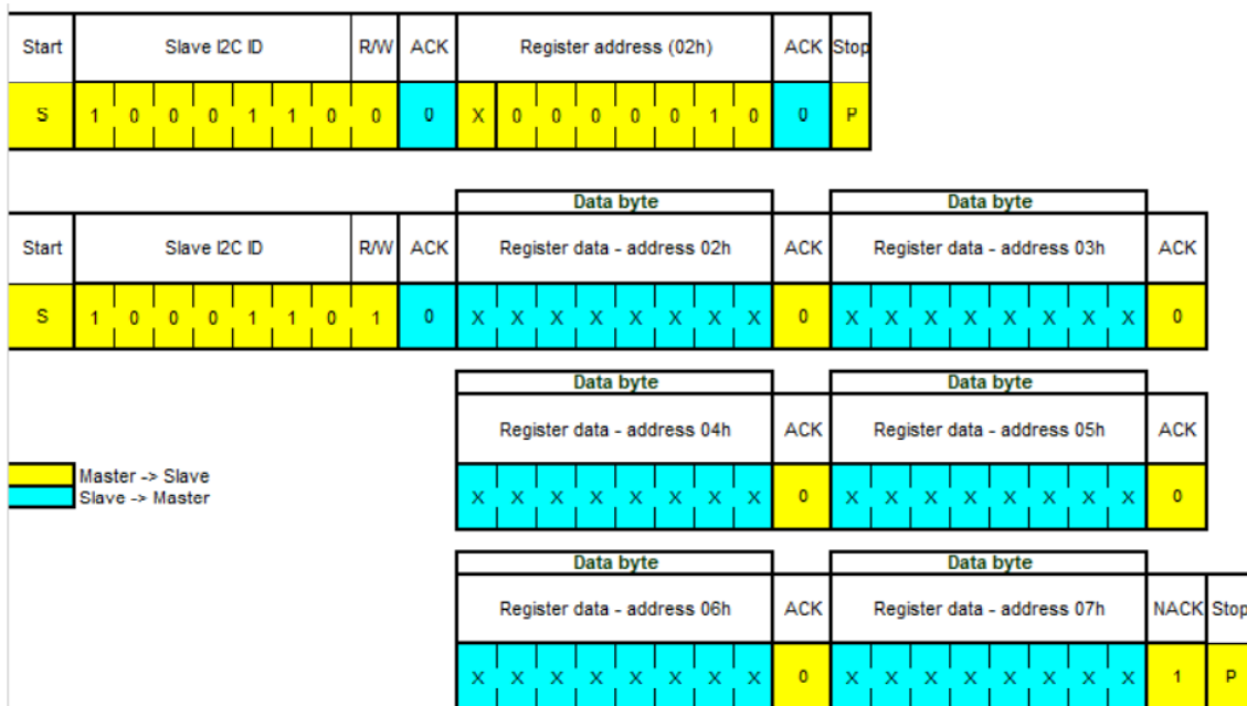
Figure 16: multi-byte read protocol with stop-start
