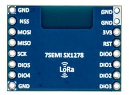
The **7Semi LoRa RA-02** module is a wireless communication module based on the **Semtech** SX1278 LoRa transceiver chip. It operates in the **433 MHz frequency band** and is widely used in long-range, low-power IoT applications. LoRa (Long Range) technology enables efficient data transmission over long distances while consuming minimal power.
